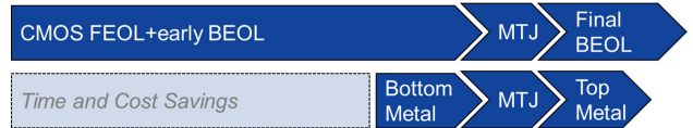
FIGURE 2. Short Flow test vehicle for memory element test enables faster learning cycle and lowers the development cost compared to full flow wafers with integrated memory process. Bottom graph shows potential time saving and impact on learning cycle of embedded memory using Short Flow approach.
